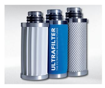
The secret of this vast increase in performance lies in the pleating of the nano-filter media. The pleating process mechanically folds the non- woven filter media many times. This makes the filter area 450% larger than that of a conventio- nal rapped filter element.
